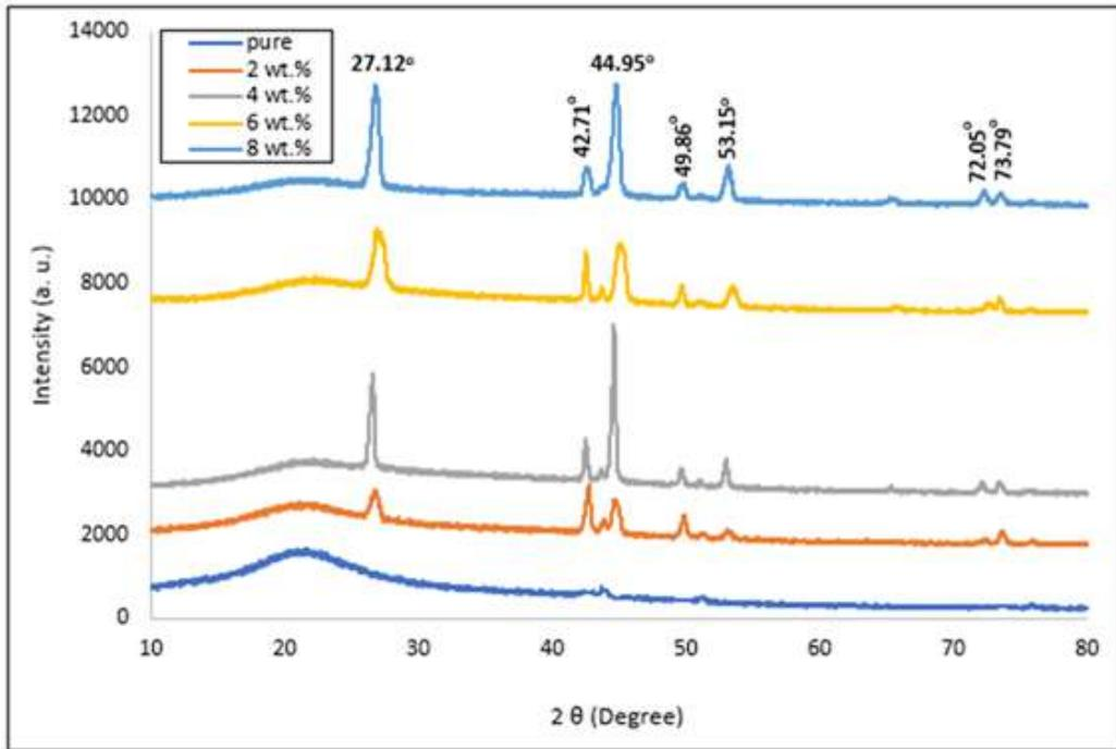
Figure 1. X-ray diffraction for (CMC/ZnSe) nanocomposites
