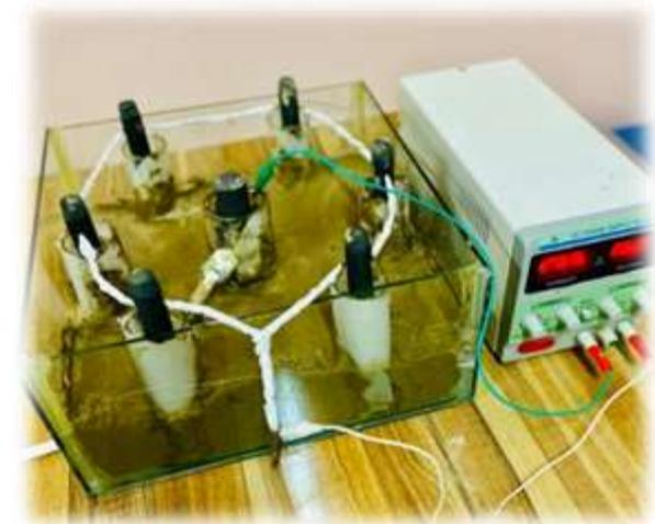
**Figure 1.** *Electrokinetic chamber experimental configuration, which consists of hexagonal-shaped anode electrodes arranged around the cathode electrode*
