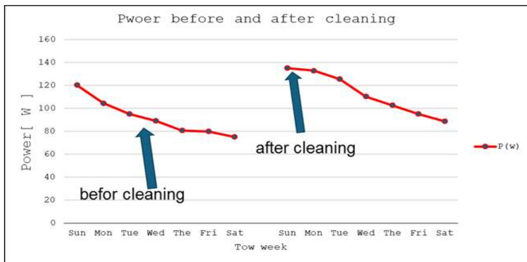
Figure 12. The output power of the photovoltaic panel is under water cleaning for 7 days without cleaning the cell itself in the second week
