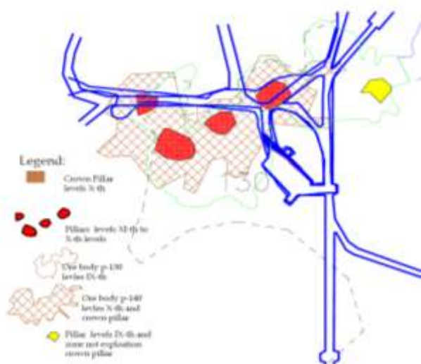
Figure 4. 9th level, P-130 ore body, crown pillar and safety pillars of 10th level
