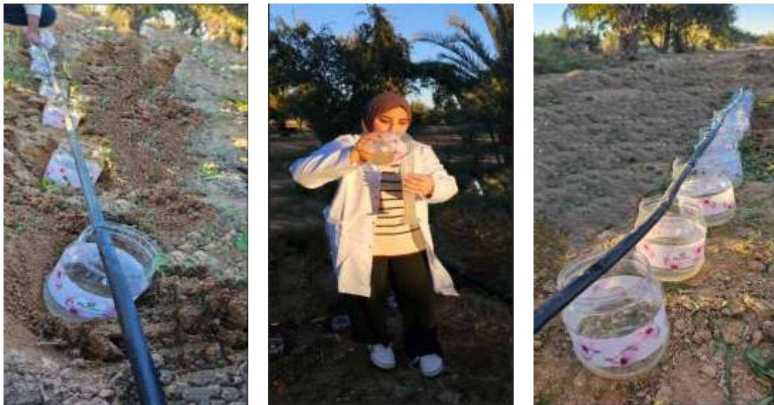
Figure 3. Process of evaluate the discharge of the drippers of the surface drip irrigation system.
