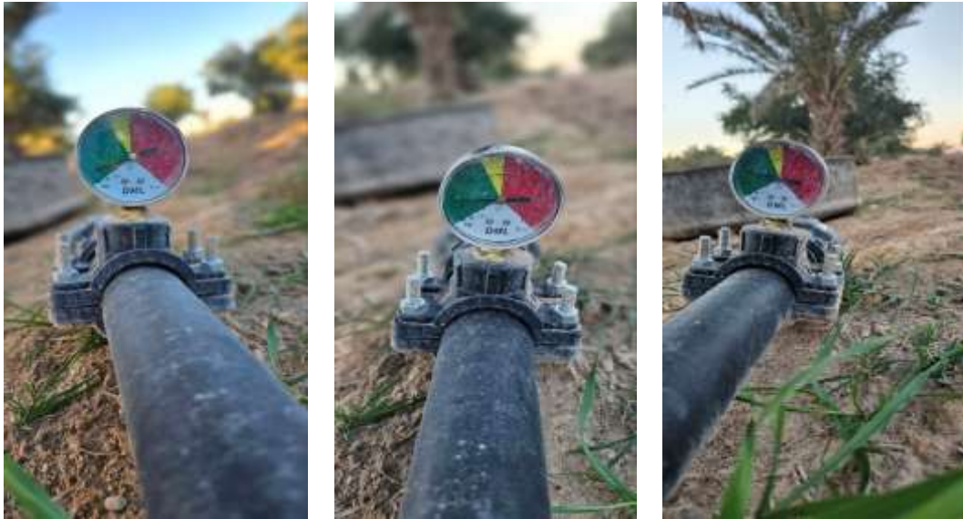
Figure 2. Different operating pressures (1bar ,1.5 bar ,2 bar) to evaluate the drainage of the drippers of the surface drip irrigation system and the uniformity of water distribution.
