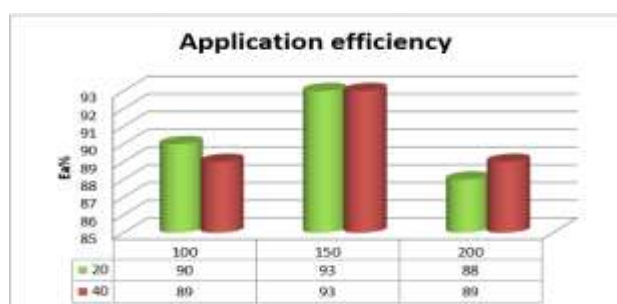
Figure 7. Application efficiency vs operating pressure for surface drip irrigation with different distance between emitters (20,40) cm.
