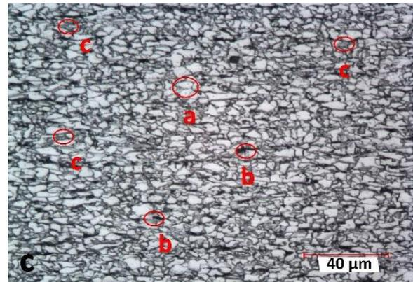
**Figure 2.** Microstructure of Nb-added microalloyed steel (EN 10149-2:2013 S355MC (QStE 380TM)) ( in figure c a : ferrite b : pearite c : NbC )
