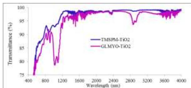
Figure 2. FT-IR Analysis of silane-based oxide coatings.
