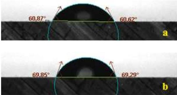
**Figure 4.** Contact angles measurements of silane based oxide coatings a) GLYMO-TiO<sub>2</sub> and b) TMSPM-TiO<sub>2</sub>.
