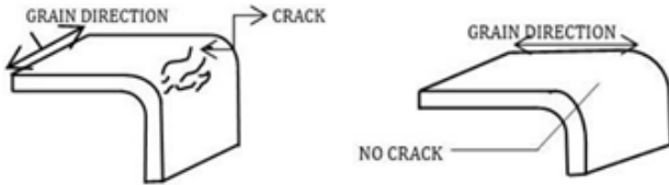
Figure 2. Example of Forming Error, Cracking [8]
