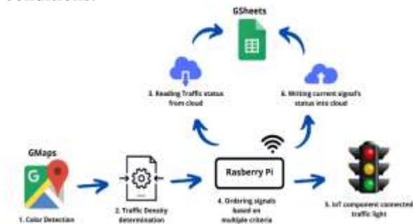
Figure 2. Intelligent Traffic Signal Management Methodology
