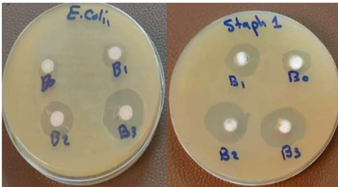
Figure 4. Image for inhibition zones unexposed pure PE and PE exposed argon with different time (10, 20 and 25) min. on S. aureus and E. coli on S. aureus and E. coli
