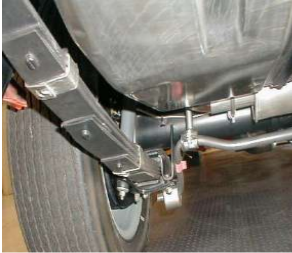
Figure 1. An arrangement of leaf springs in the traditional fashion [7].
