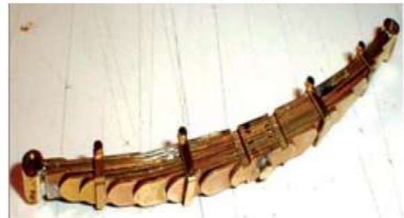
Figure 4. Form a graduated or laminated leaf spring.
