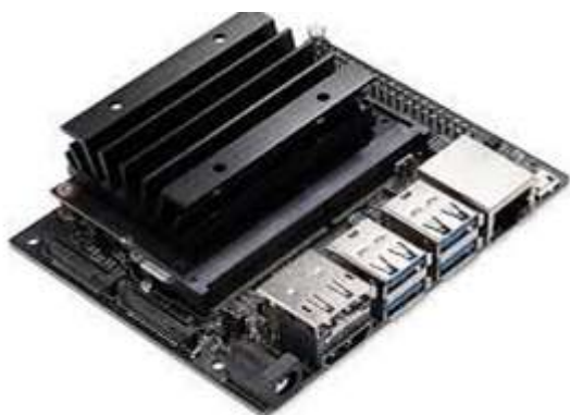
Figure 4. NVIDIA Jetson Nano Board Version-2 used as the Edge Gateways
