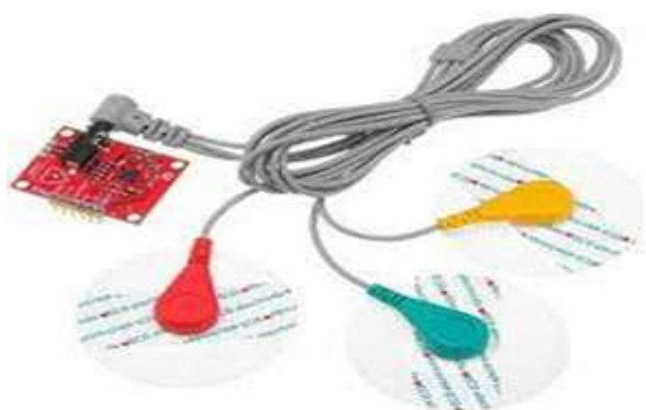
Figure 2. ECG Sensors with the Three Electrodes used in the Proposed research
