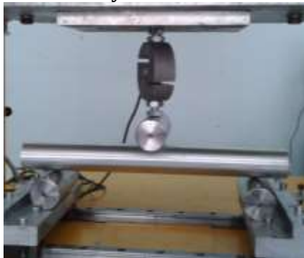
Figure 1. a) Experimental set-up for three-point bending validation test, b) Finite element analysis model
