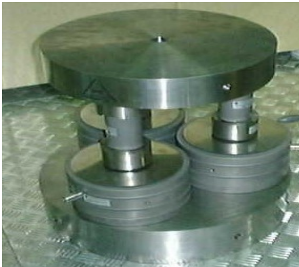
Figure 9. Combining three 1 MN force transducers for 3 MN built-up transducers
