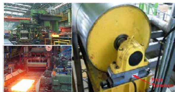
Figure 6. Rolling force measuring equipment
