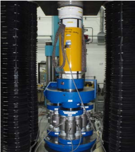
Figure 10. Calibration of 5 MN single force transducer using 9x540 kN built-up transducer [NPL]
