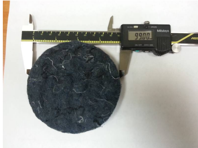
Figure 3. Measurement of test specimens dimensions by caliper
