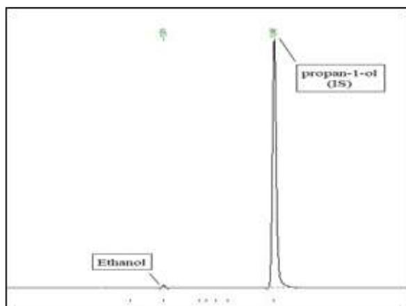
**Figure 1.** The chromatogram of ethanol (RT:1.01min.) at a concentration of 4.0 mg/dL and IS (RT:1.68 min)
