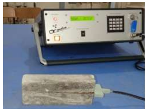
Figure 6. Device of Thermal conductivity-meter
