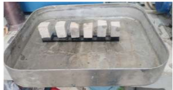
Figure 5. Water absorption by capillary test
