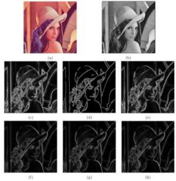
Figure 1. Comparison of different edge detection methods: (a) original image; (b) grayscale image, (c), (d) and (e) are obtained by using Sobel, Canny and Prewitt filters, respectively; (f), (g) and (h) are obtained by using (2) for \alpha = 0.25, 0.75 and 0.99 , respectively
