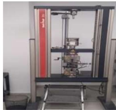
Figure 2: Zwick Roell Z050 Tensile Test Machine
