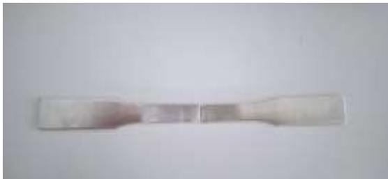
**Figure 6:** Sample after tensile test.
