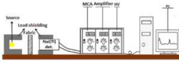
**Figure 1.** Schematic view of the gamma spectroscopy system (Akkurt et al., 2015)
