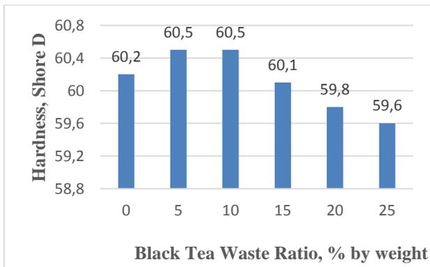
Figure 6. Variation of Shore D Hardness Value with Black Tea Waste Ratio
