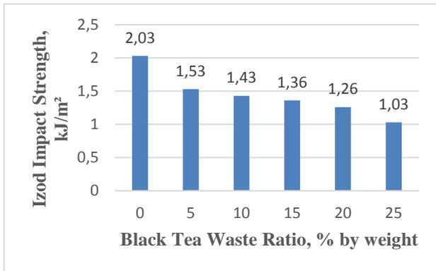
Figure 5. Variation of Izod Impact Strength with Black Tea Waste Rate
