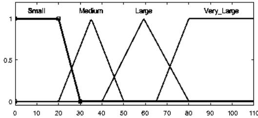
Figure 6. Membership functions for "PV"
