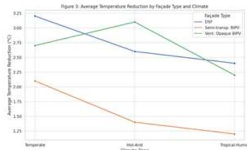
Figure 3. Average Temperature Reduction by Façade Type and Climate
