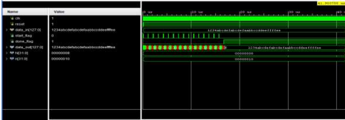
Figure 5: UART - Simulation Waveform for Extension Paper
