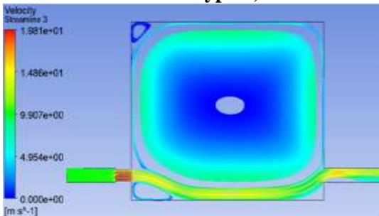
e. Velocity Stream line contour in m/s (without bypass)
