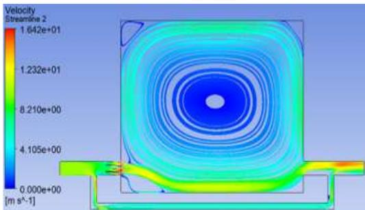
e. Velocity Stream line contour in m/s for triangular nozzle
