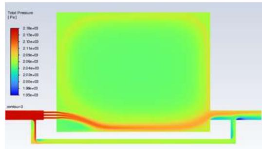
d. Pressure contour in pa for rectangular nozzle
