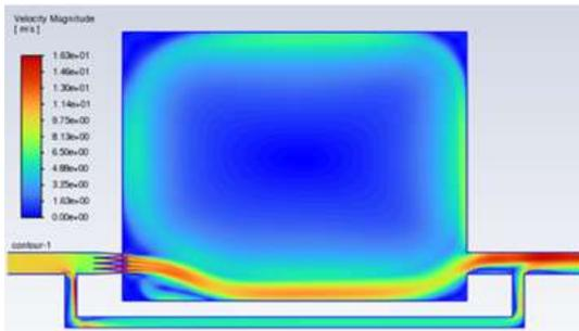
a. Velocity magnitude in m/s for triangular nozzle
