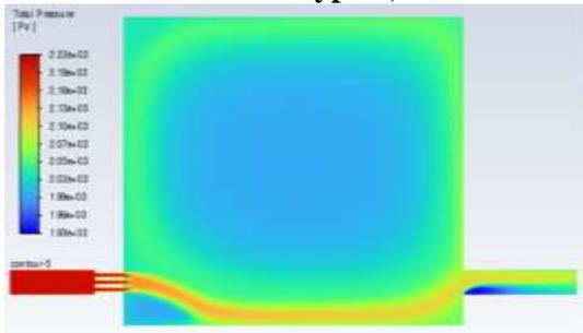
c. Pressure contour in pa (Without bypass)
