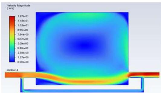
a. Velocity magnitude in m/s for 1800 pa suction pressure
