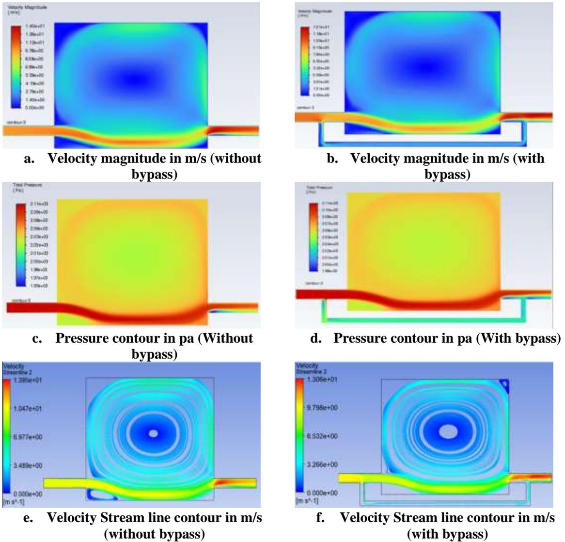
Figure. 1. a to f represents Velocity, Pressure, and Streamline Contours (With and Without Bypass) without a nozzle.
