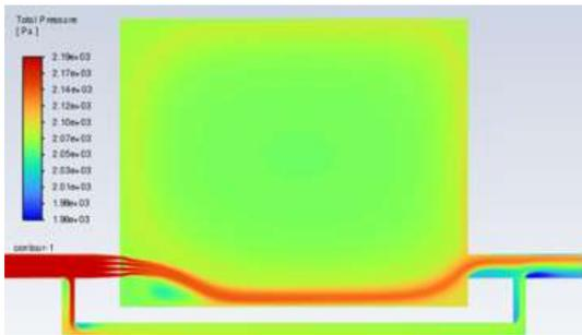
c. Pressure contour in pa for triangular nozzle
