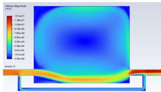
b. Velocity magnitude in m/s for 1600 pa suction pressure
