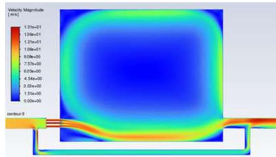
b. Velocity magnitude in m/s (with bypass)
