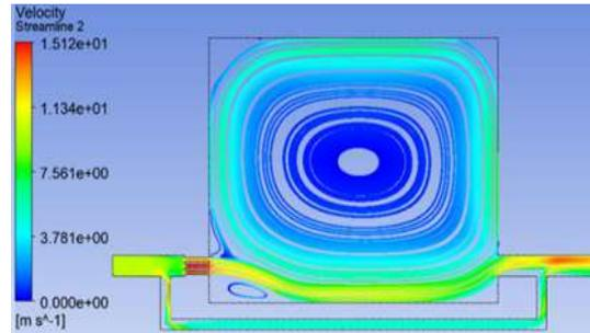
f. Velocity Stream line contour in m/s (with bypass)
