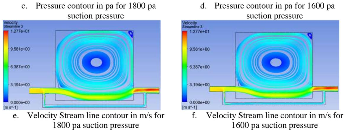
**Figure 4.** a,c,e and b,d,f represent Velocity, Pressure, and Streamline for 1800 and 1600 pa suction pressure respectively
