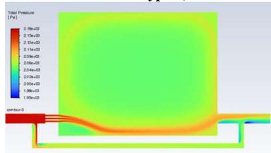
d. Pressure contour in pa (With bypass)
