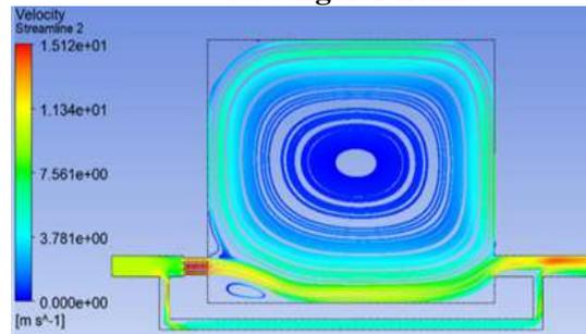
f. Velocity Stream line contour in m/s for rectangular nozzle
