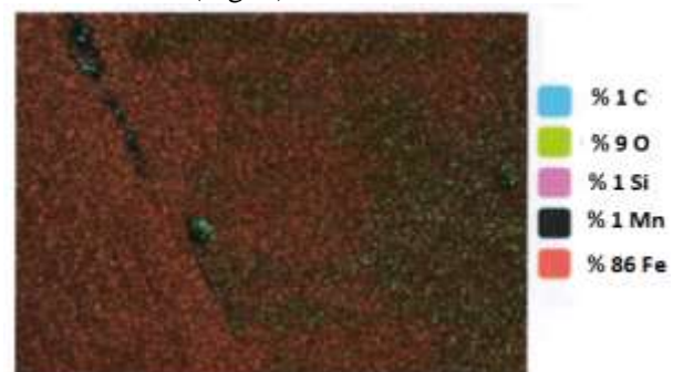
Figure 3. Chemical compositions of base metal region of S420MC DP steel welded with RSW
