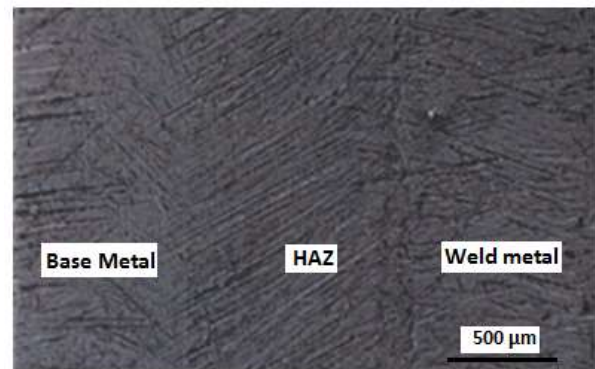
Figure 2. SEM micrograph of S420MC DP steel welded with RSW method.
