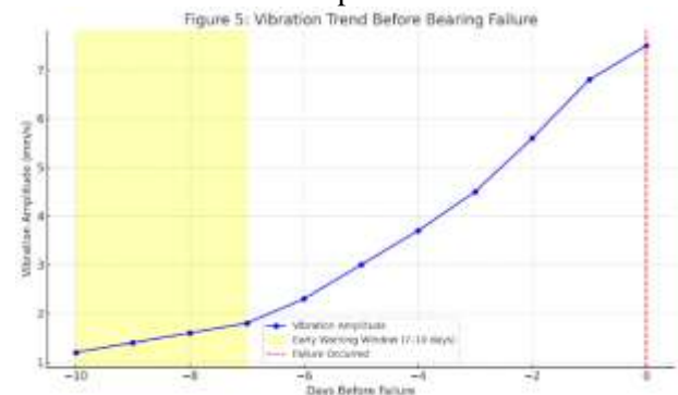
Figure.3: Time-series trend of vibration amplitude in an industrial motor, illustrating early warning signals 7–10 days prior to bearing failure
