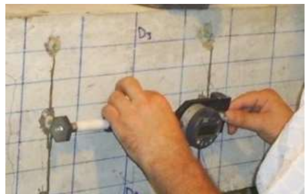
Figure 7. Mechanical extensometer with digital reader
