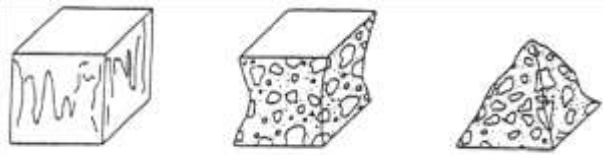
Figure 2. Process of testing the compressive strength of concrete
