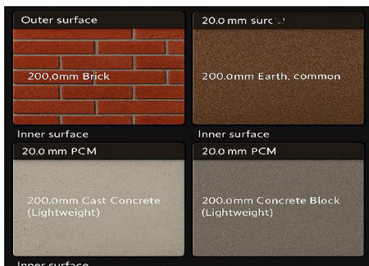
Figure 4. Wall envelope PCM integration configurations. Source: Author
