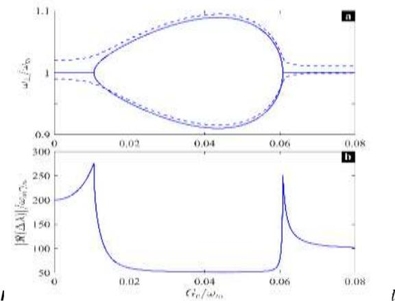
sensitivity after a perturbation (dashed curve) in presence of the BSBS process. The perturbation strength is  $\epsilon = 10^{-2}\omega_m$  and the other parameters are the same as those in **Figure 2**.
