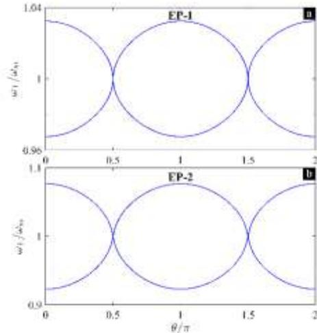
**Figure 3.** Eigenfrequencies versus the phase  $\theta$  for (a) EP-1 at  $G_c = 0.01049\omega_m$  and (b) EP-2 at  $G_c = 0.06110\omega_m$ , in presence of the BSBS process ( $G_b = 10^{-2} \omega_m$ ). The used parameters are the same as those in Figure 2.
