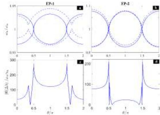
**Figure 5.** (a) Eigenfrequencies splitting and (b) the resulted sensitivity after a perturbation (dashed curve) at EPs, in presence of the BSBS process. The other parameters are the same as those in **Figure 2**.
