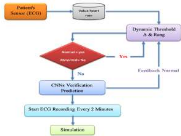
Figure 1. Flowchart of the Dynamic Threshold Proposed System.
