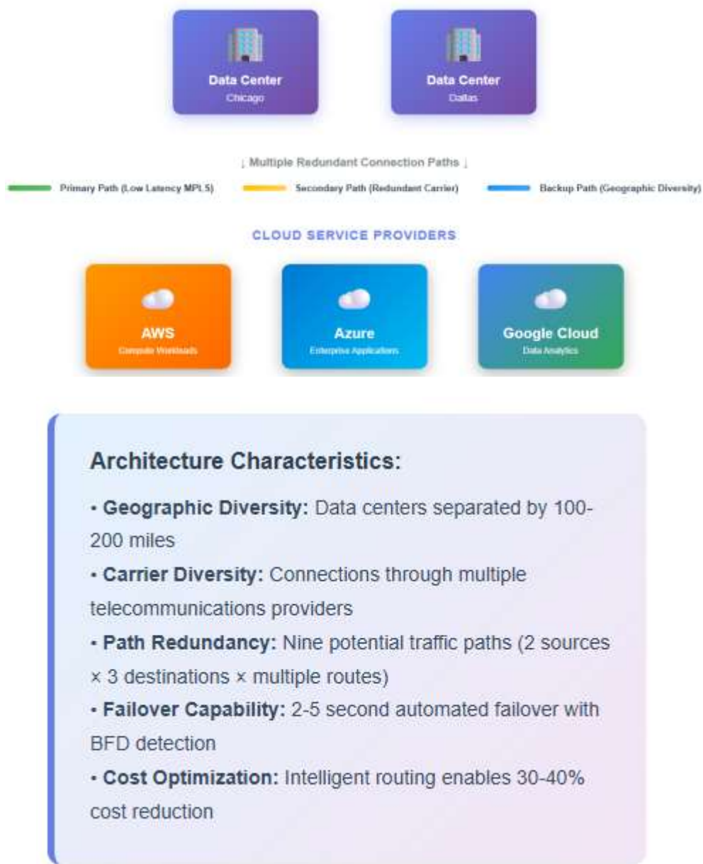
Figure 1: Multi-Cloud Connectivity Architecture with Redundant Paths.
