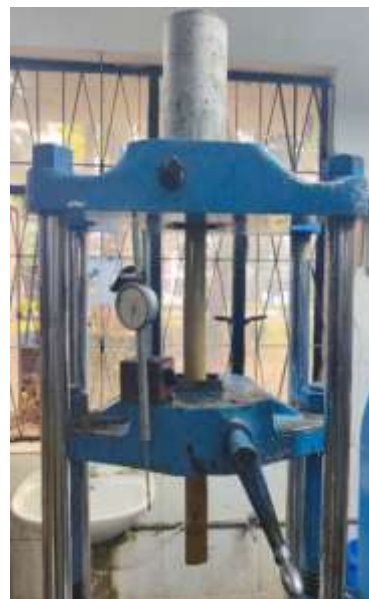
Figure 3. Loading setup for pull-out test [21].
