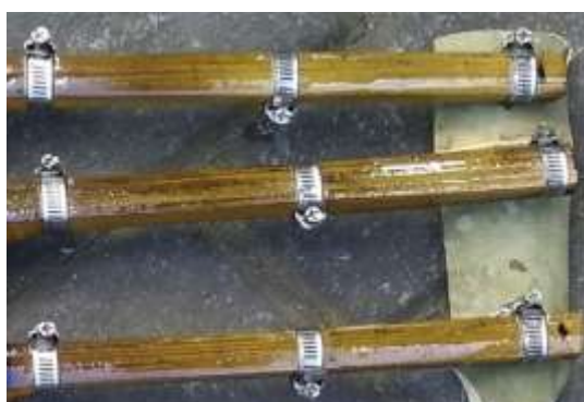
Figure 9. Bamboo with hose clamps and layer of Sikadur-752 [31]
