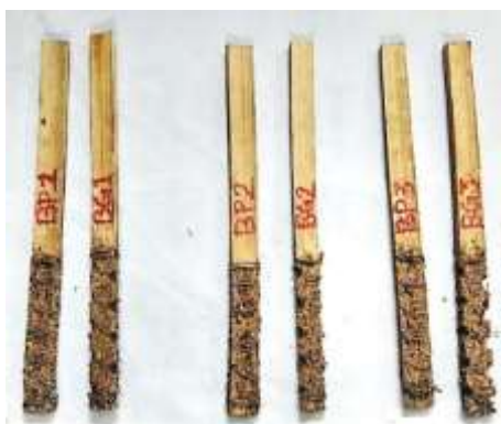
Figure 7. Bamboo specimens with Bond tite coating and sand particles [16].
