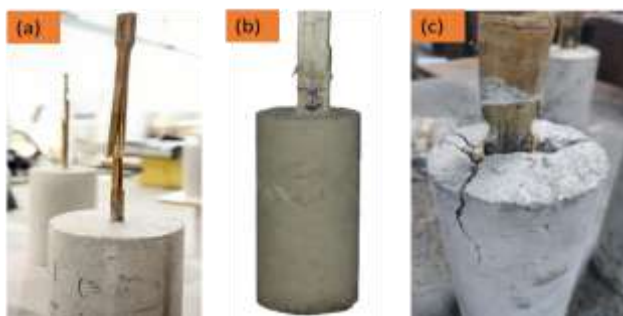
Figure 11. Failure modes observed during pull-out test (a) Tensile failure of bamboo [33] (b) Slippage of bamboo [30] (c) Bond failure with concrete splitting [21]
