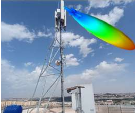
Figure 2. Electrical tilt configuration of the RRV4-65D-R6 antenna.
