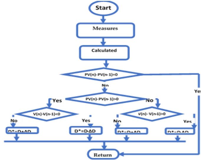
Figure 2. Flowchart of P&O MPPT algorithm [15]
