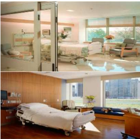
Figure 2. The difference in glare and light reflection. On the right is an example of glossy floors and on the left is a matte floor [14].
