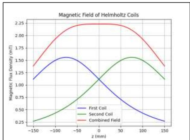
Figure 5. Magnetic Field of the Helmholtz Coils as a combination of the fields of each coil
