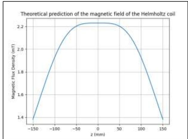
Figure 3. Theoretical prediction of the magnetic field of the Helmholtz coil with 124 turns and current 3A.
