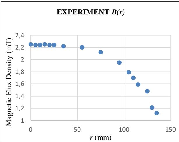
Figure 7. Experimental Measurement of Magnetic Flux Density ( $B$ ) vs. Radial Distance ( $r$ ) for Helmholtz Coil.
