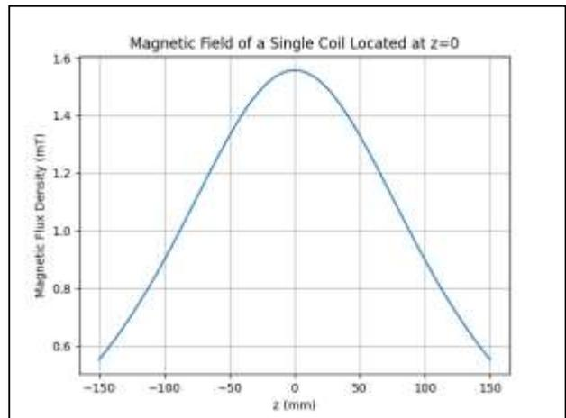
Figure 4. Theoretical prediction of the magnetic field of one coil with 124 turns and current 3A.
