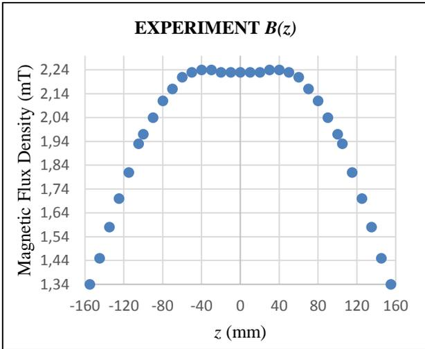
Figure 6. Experimental Measurement of Magnetic Flux Density vs. Distance ( $z$ -Axis) for Helmholtz Coil.
