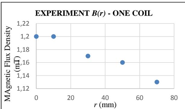
Figure 8. Experimental Measurement of Magnetic Flux Density ( $B$ ) vs. Radial Distance ( $r$ ) for a Single Coil.
