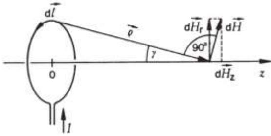
Figure 1. Drawing for the calculation of the magnetic field along the axis of a wire loop. (PHYWE)
