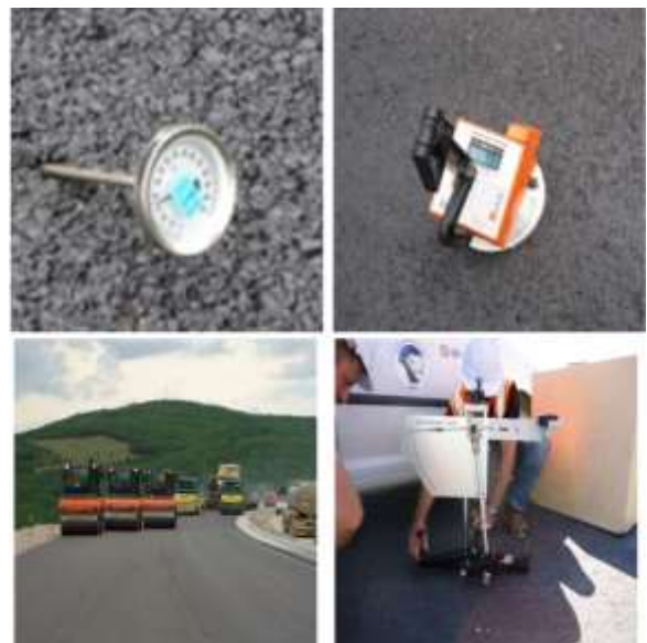
Figure 4. Measurement of asphalt temperature before asphaltting, measurement of compaction rate by non-destructive method, compaction phases, determination of skid resistance
