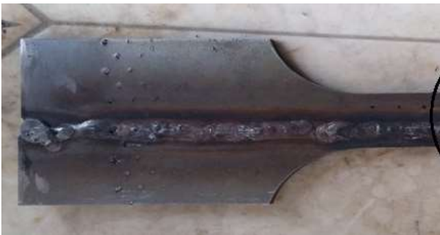
Figure 3. A photograph of the failure point in AISI 430 ferritic stainless steel welded using the TIG process.
