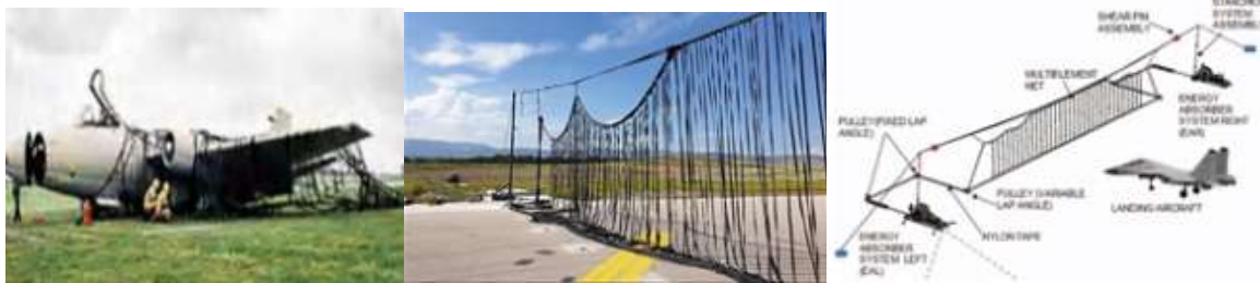
Figure 2: Net type AAS barrier system.
