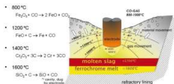
Figure 1. Reaction zones in an electric arc furnace [13, 14]
