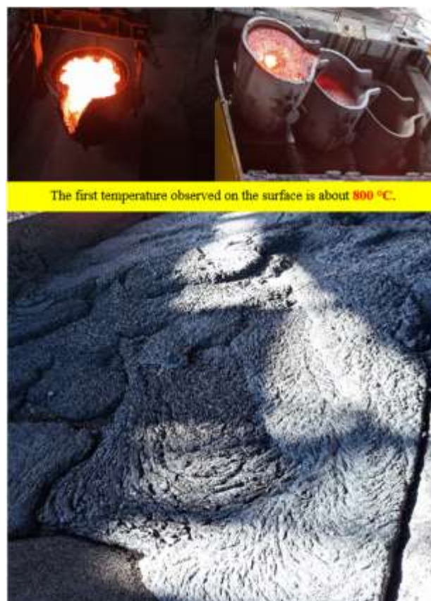
Figure 3. HC FeCr production in EAF of Eti Krom Inc.
