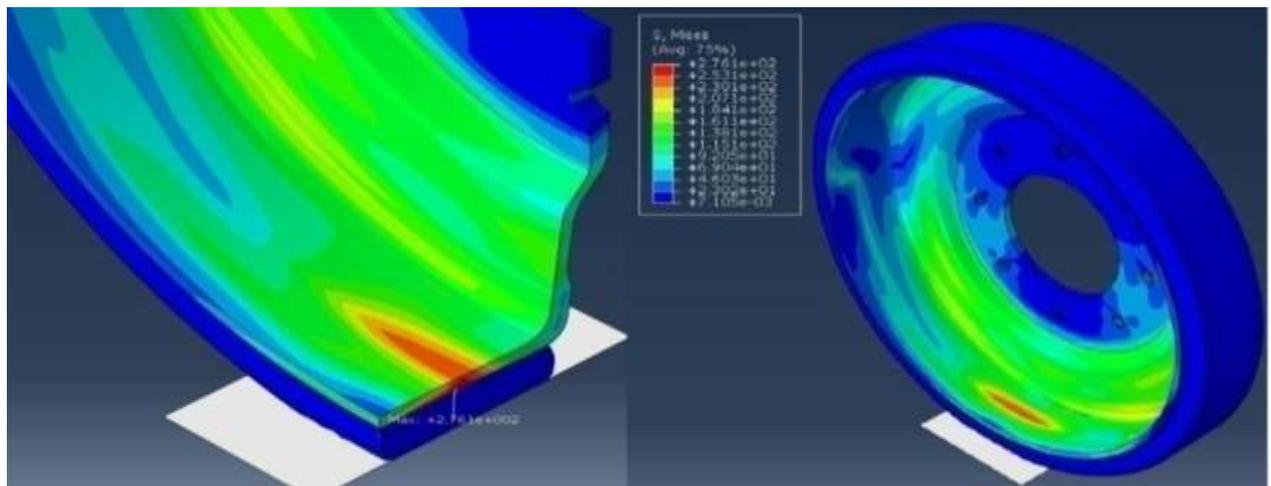
Figure 12. Maximum stress on the Road Wheel rim when a 20x25x20 mm reinforcement ring is used. (Reinforcement Ring is hidden.)
