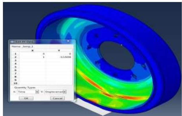
Figure 16. Road wheel with welded wear plate without reinforcement ring.
