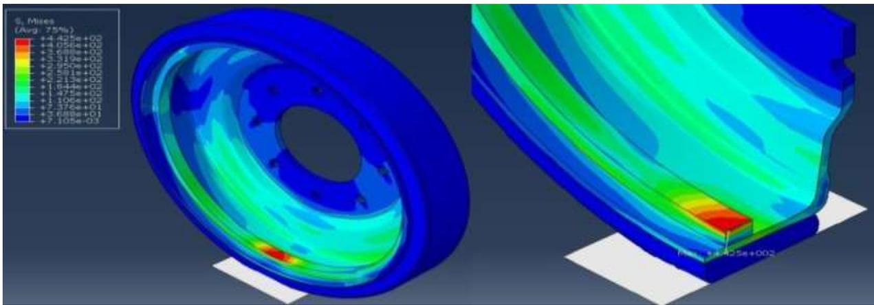
Figure 11. Maximum stress on the reinforcement ring with dimensions of 20x25x20 mm.
