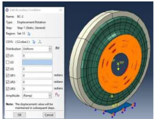
Figure 7. Finite element model boundary conditions
