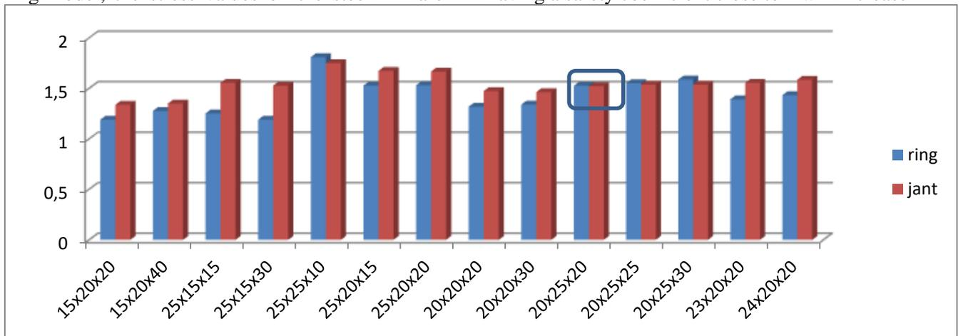
**Figure 10. Safety coefficient on the reinforced ring and steel rim mounted in various sizes.**
