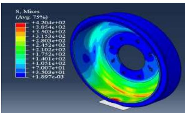
**Figure 8.** Road Wheel made of SAE 3957 material without reinforcement hoop
