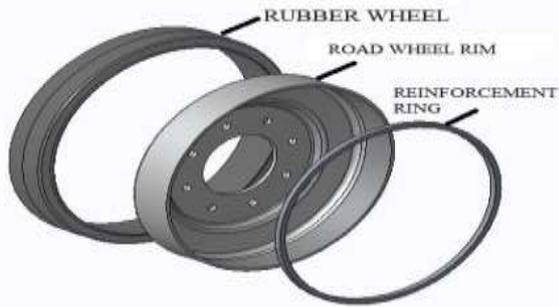
Figure 2. Creo Parametric Modeling of the Components of the Road Wheel.
