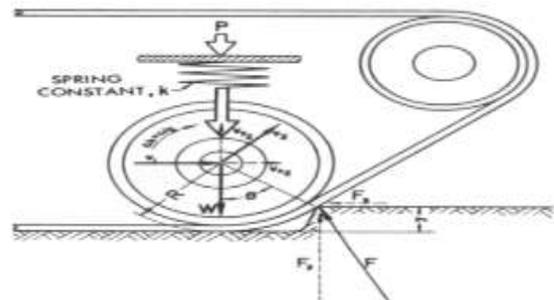
Figure 3: Impact Force Components on the Road Wheel.
