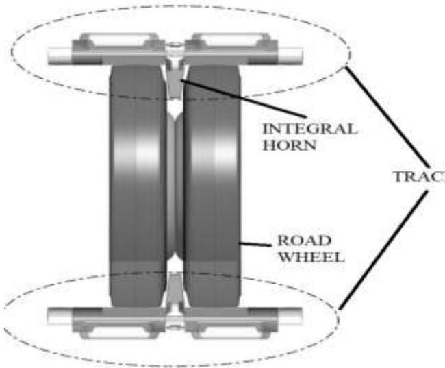
Figure 13. Pallet link working with road wheel
