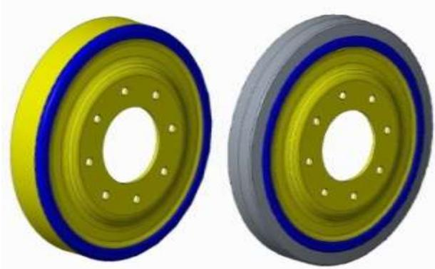
Figure 14. Road wheel with wear plate welded on
