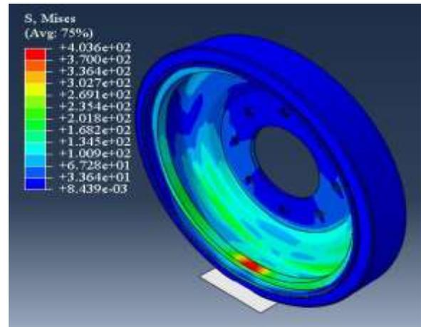
Figure 15: Maximum stress on the Wear Plate Road Wheel
