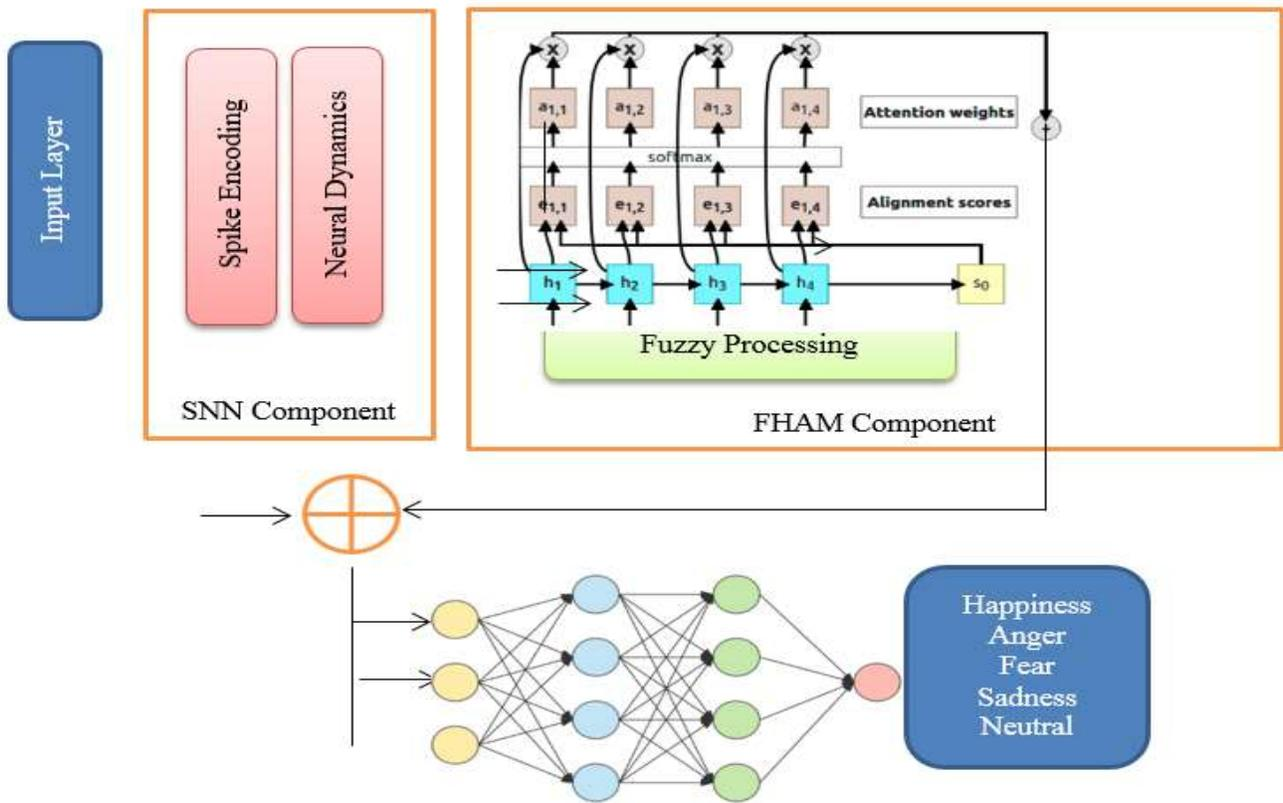
Figure 2. An architecture of the NeuroFuzzy SpikeNet
