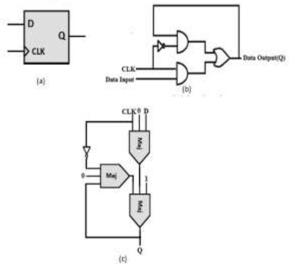
Figure 7. Proposed Designs of D type Flip-flop (a) Pictogram (b) Circuit Diagram using logic gates (c) Circuit diagram using Majority Gates.
