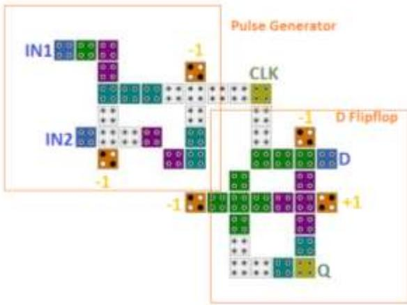
Figure 8. Suggested QCA layout for D FF with pulse generator.
