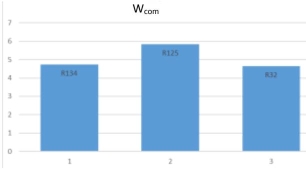
Figure 12. Work (electricity) values consumed on the compressor obtained as a result of calculations for R32, R125 and R134 working fluids of the analysed ground source heat pump
