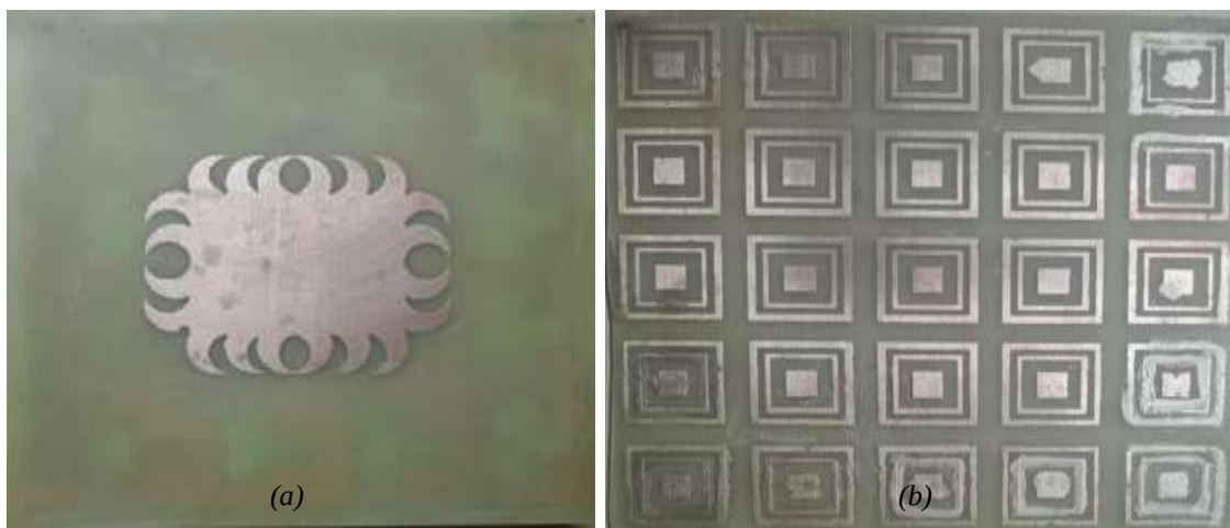
Figure 6. Proposed fabricated models (a) antenna (b) AMC surface
