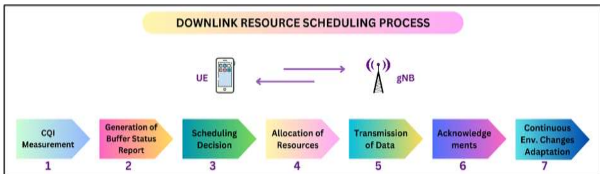
Figure 2. The downlink scheduling procedure
